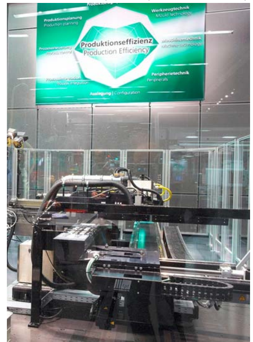
Production efficiency through process integration: At the Fakuma 2012, Arburg is presenting a production cell with inline printing for the manufacture of individually decorated plastic parts.
